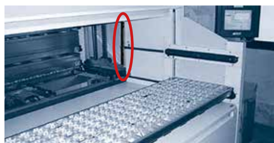
Measurement light curtains location
