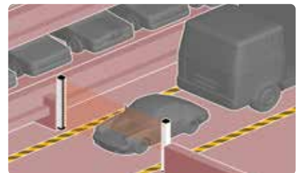
Detection of overall dimensional limits of vehicles for vehicle handling in automatic parking garages
